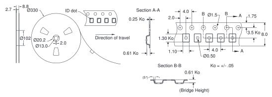
Standard T/R size=15,000 units/reel. All dimensions are in millimeters.
