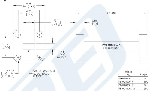
WR-28 Instrumentation Grade Straight Waveguide Section 12 Inch Length with 599/U Flange Operating from 26.5 GHz to 40 GHz from Pasternack Enterprises has same day shipment for domestic and International orders. Our RF, microwave and millimeter wave products maintain a 99% availability and are part of the broadest selection in the industry.
