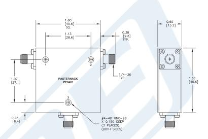
50 Ohm SMA Circulator Operating From 2 GHz to 4 GHz And 10 Watts With 18 dB Isolation from Pasternack Enterprises has same day shipment for domestic and International orders. Our RF, microwave and fiber optic products maintain a 99% availability and are part of the broadest selection in the industry.
