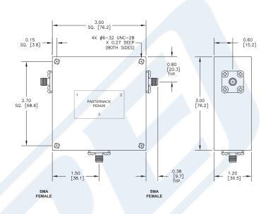
50 Ohm SMA Circulator Operating From 135 MHz to 175 MHz And 150 Watts With 20 dB Isolation from Pasternack Enterprises has same day shipment for domestic and International orders. Our RF, microwave and millimeter wave products maintain a 99% availability and are part of the broadest selection in the industry.
