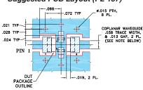
COPLANAR WAYEGUIDE PARAMETERS ARE SHOWN FOR ROGERS ROA\$50B WITH THICKNESS .020" ± .0015". COPPER: 1/2 02. EACH SIDE. FOR OTHER MATERIALS TRACE WIDTH & GAP MAY NEED TO BE MODIFIED.
