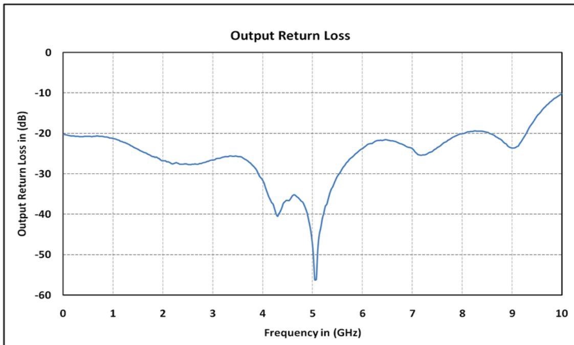
**Test fixture data***Driver Bias +5V,-5V; Control 0/+5V;  $T_A = 25^\circ\text{C}$*
