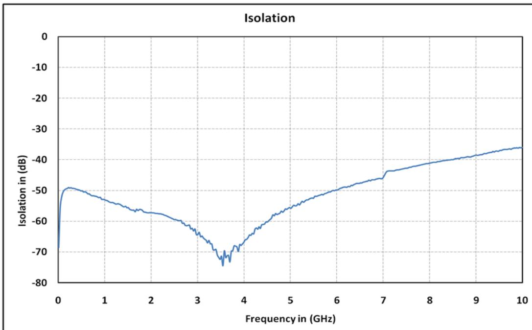
**Test fixture data***Driver Bias +5V,-5V; Control 0/+5V;  $T_A = 25^\circ\text{C}$*
