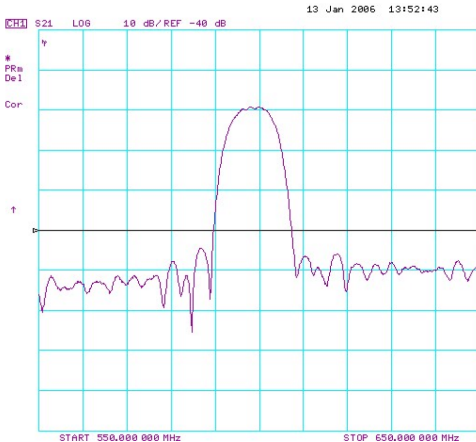
Fig-1 S21 Response Horizontal: 10MHz/Div Vertical: 10dB/Div
