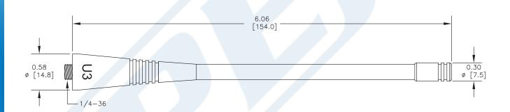
Click the following link (or enter part number in "SEARCH" on website) to obtain additional part information including price, inventory and certifications: Whip Antenna Operates From 450 MHz to 470 MHz With a Typical 0 dBi Gain SMA Female Input Connector IP67 Rated PE51148
