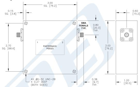
50 Ohm SMA Isolator Operating From 330 MHz to 403 MHz And 150 Watts With 20 dB Isolation from Pasternack Enterprises has same day shipment for domestic and International orders. Our RF, microwave and millimeter wave products maintain a 99% availability and are part of the broadest selection in the industry.
