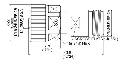
Note: NMD 3.5 Jack to be mounted directly on vector network analyser.
