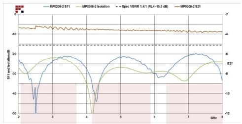
2 Way Power Divider SMA Connectors From 2 GHz to 8 GHz Rated at 30 Watts from Fairview Microwave is in-stock and available to ship same-day. All of our RF/microwave products are available off-the-shelf from our ISO 9001:2008 certified facilities in Allen, Texas. Fairview Microwave is RF on-demand.
