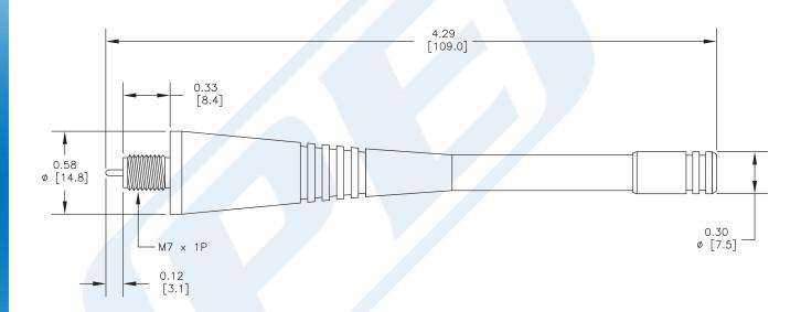
Click the following link (or enter part number in "SEARCH" on website) to obtain additional part information including price, inventory and certifications: Whip Antenna Operates From 698 MHz to 870 MHz With a Typical 2 dBi Gain MD Male Input Connector IP67 Rated PE51150
