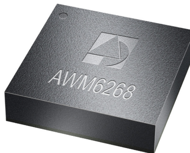
10 Pin 4 mm x 4 mm x 1 mm Surface Mount Module
