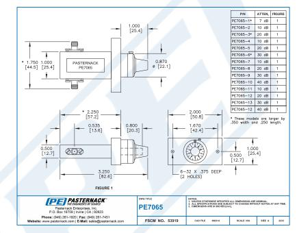
0 to 40 dB Rotary Continuously Variable Attenuator, SMA Female To SMA Female Rated To 5 Watts From 12.4 GHz To 18 GHz from Pasternack Enterprises has same day shipment for domestic and International orders. Our RF, microwave and millimeter wave products maintain a 99% availability and are part of the broadest selection in the industry.
