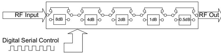
The DAT-15R5A-SN+ serial interface consists of 5 control bits that select the desired attenuation state, as shown in Table 1: Truth Table
