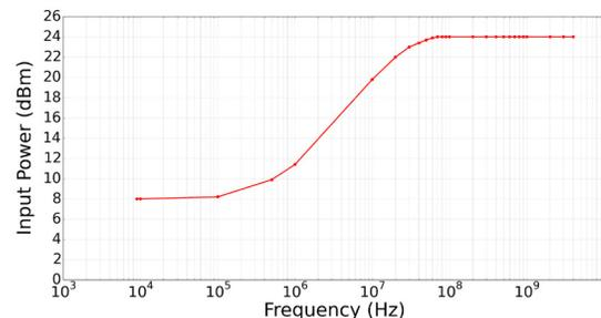
Figure 1. Max Input Operating Power vs Frequency
