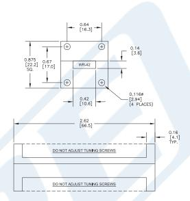
Bandpass Waveguide Filter With WR-42 Interface And a Pass Band From 20.2 GHz to 21.2 GHz from Pasternack Enterprises has same day shipment for domestic and International orders. Our RF, microwave and millimeter wave products maintain a 99% availability and are part of the broadest selection in the industry.
