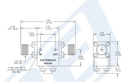
50 Ohm SMA Isolator Operating From 8 GHz to 18 GHz And 1 Watts With 16 dB Isolation from Pasternack Enterprises has same day shipment for domestic and International orders. Our RF, microwave and fiber optic products maintain a 99% availability and are part of the broadest selection in the industry.
