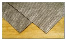
MAC-2100-WP is a simple solution for effective RF signal attenuation in many commercial applications. It provides –100 dB <u>RF isolation from 100 MHz to 1 GHz and more than -70 dB to</u> <u>18GHz</u>. Very light, thin, flexible, wear and tear resistant, it can be applied directly to studs, standard sheetrock and other structures using simple and inexpensive methods. The product is well suited to both new and retrofit construction. It provides a good degree
