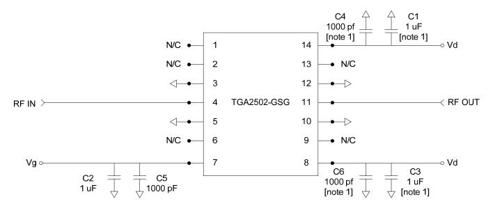
Note 1: Remove cap for pulsed drain operation
