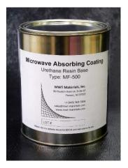
MF-500 broadband MagRAM coating is a coated carbonyl iron based paint in a proprietary urethane acrylic resin. It provides broadband RF absorption with a thin format. Its durable abrasion resistant finish is stable in hot and cold environments. The product can be applied with a brush or Sprayer. It has excellent UV Resistance. A marine grade is also available.
