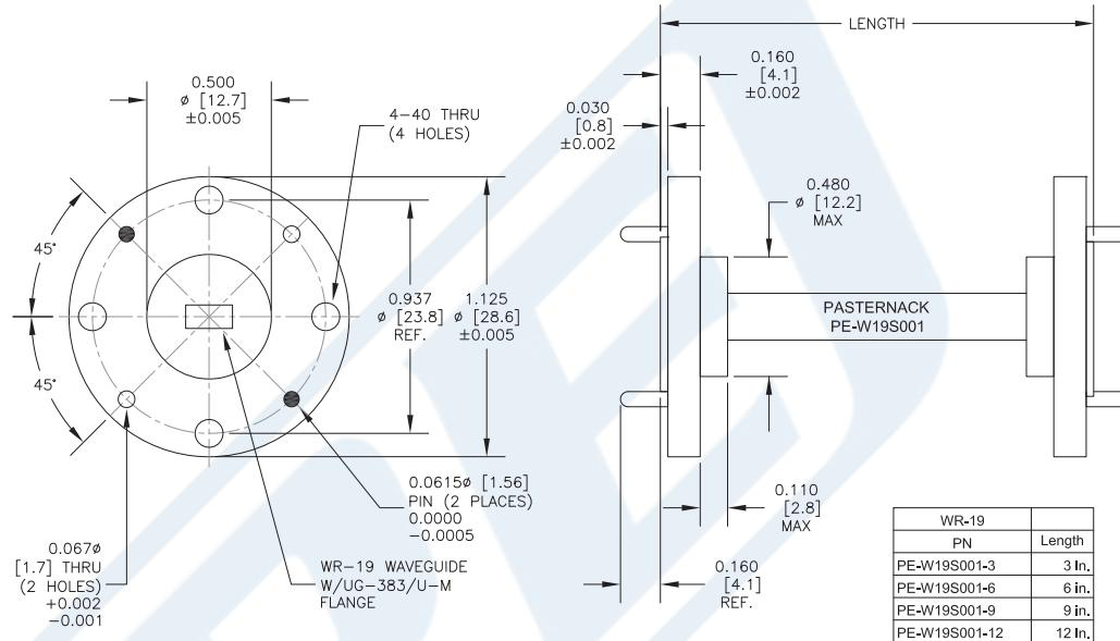
WR-19 Instrumentation Grade Straight Waveguide Section 6 Inch Length with UG383/U-Mod Flange Operating from 40 GHz to 60 GHz from Pasternack Enterprises has same day shipment for domestic and International orders. Our RF, microwave and millimeter wave products maintain a 99% availability and are part of the broadest selection in the industry.
