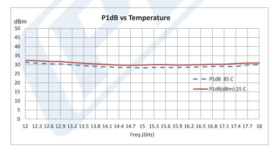
Click the following link (or enter part number in "SEARCH" on website) to obtain additional part information including price, inventory and certifications: 1 Watt, 12 GHz to 18 GHz, Medium Power Broadband Amplifier, 33 dB Gain, 39 dBm IP3, 6 dB NF, SMA PE15A4002
