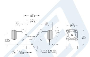
50 Ohm N Isolator Operating From 4 GHz to 8 GHz And 10 Watts With 18 dB Isolation from Pasternack Enterprises has same day shipment for domestic and International orders. Our RF, microwave and fiber optic products maintain a 99% availability and are part of the broadest selection in the industry.
