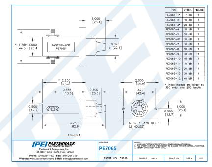
0 to 30 dB Rotary Continuously Variable Attenuator, SMA Female To SMA Female Rated To 5 Watts From 4 GHz To 8 GHz from Pasternack Enterprises has same day shipment for domestic and International orders. Our RF, microwave and millimeter wave products maintain a 99% availability and are part of the broadest selection in the industry.
