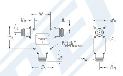
50 Ohm N Circulator Operating From 698 MHz to 960 MHz And 1000 Watts With 18 dB Isolation from Pasternack Enterprises has same day shipment for domestic and International orders. Our RF, microwave and fiber optic products maintain a 99% availability and are part of the broadest selection in the industry.
