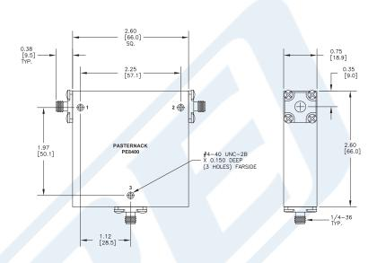
50 Ohm SMA Circulator Operating From 1 GHz to 2 GHz And 10 Watts With 18 dB Isolation from Pasternack Enterprises has same day shipment for domestic and International orders. Our RF, microwave and fiber optic products maintain a 99% availability and are part of the broadest selection in the industry.
