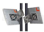
This WiFi antenna features a heavy-duty UV-stable white fiberglass radome for all-weather operation. The HG5419P antenna is supplied with a tilt and swivel mast mount kit. This allows installation at various degrees of incline for easy alignment. It can be installed for vertical or horizontal polarization.
