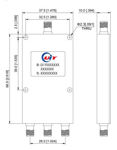
Unit: mm/ inch, General part tolerance is ±0.2mm unless otherwise stated.
