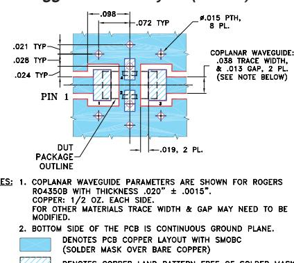
NOTES: 1. COPLANAR WAVEGUIDE PARAMETERS ARE SHOWN FOR ROGERS RO4350B WITH THICKNESS ".020" ± .0015". COPPER: 1/2 OZ. EACH SIDE. FOR OTHER MATERIALS TRACE WIDTH & GAP MAY NEED TO BE MODIFIED.
