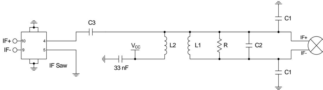
L1, C1, C2, and R form a current combiner which performs a differential to single-ended conversion at the IF frequency and sets the output impedance. In most cases, the resonance frequency is independent of R and can be set according to the following equation:
