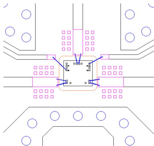
Note: MMIC die is mounted directly to carrier plate in the cutout of the EVB.
