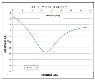
ELECTRICAL PERFORMANCE: The performance plot shown above illustrates the reflection loss performance of this material. Reflection loss is measured on a NRL arch, for more information on the NRL arch test set-up, please contact a WRS technical representative. Additional electrical test data may be available upon request.
