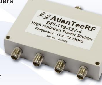
These High Isolation Power Dividers incorporate ferrite junction isolators within the branches of a Wilkinson divider structure to provide greater than 40dB isolation between output channels, combined with excellent VSWR.
