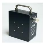
Whether for production or in the field, our low PIM loads excel. These loads are especially developed for challenging test & measurement applications, that demand accuracy and repeatability. PLOAD100 is used in production and for long duration PIM test runs. This 100W load offers PIM ratings better than -165dBc @2x43dBm. It comes with DIN 7/16 (f) connector and has a convenient carrying handle. AWT Global's PLOAD100 loads are appreciated by customers for their reliability and stable performance.
