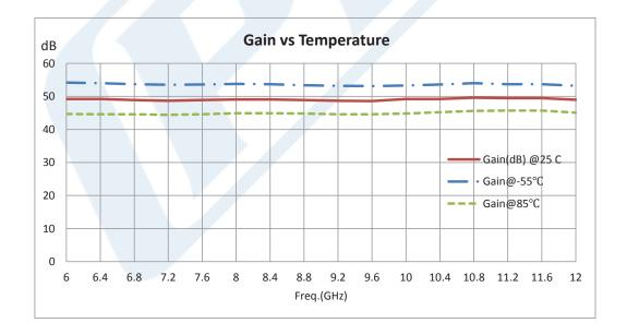
Click the following link (or enter part number in "SEARCH" on website) to obtain additional part information including price, inventory and certifications: 48 dB Gain, 1 Watt, 6 GHz to 12 GHz, Broadband High Gain Amplifier, 39 dBm IP3, 5 dB NF, SMA PE15A3505
