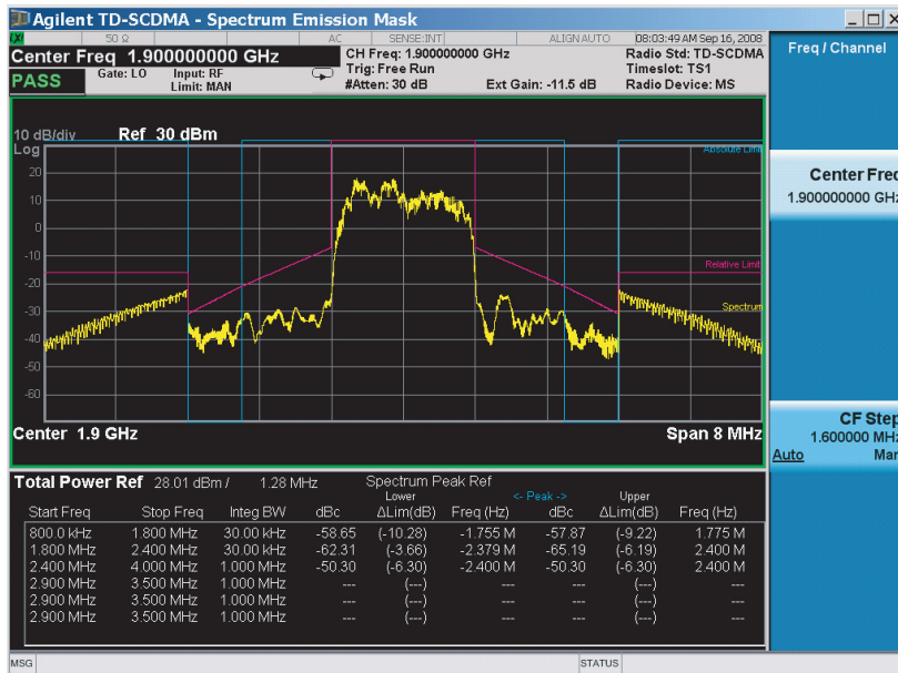
Fig 5: Spectrum Emission Mask @ 2.01GHz (Freq = 1900 MHz, P OUT = 28 dBm, V CC = 3.4 V, T c = 25 °C)
