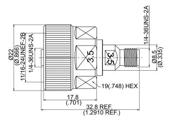
Note: NMD 3.5 Jack to be mounted directly on vector network analyser.
