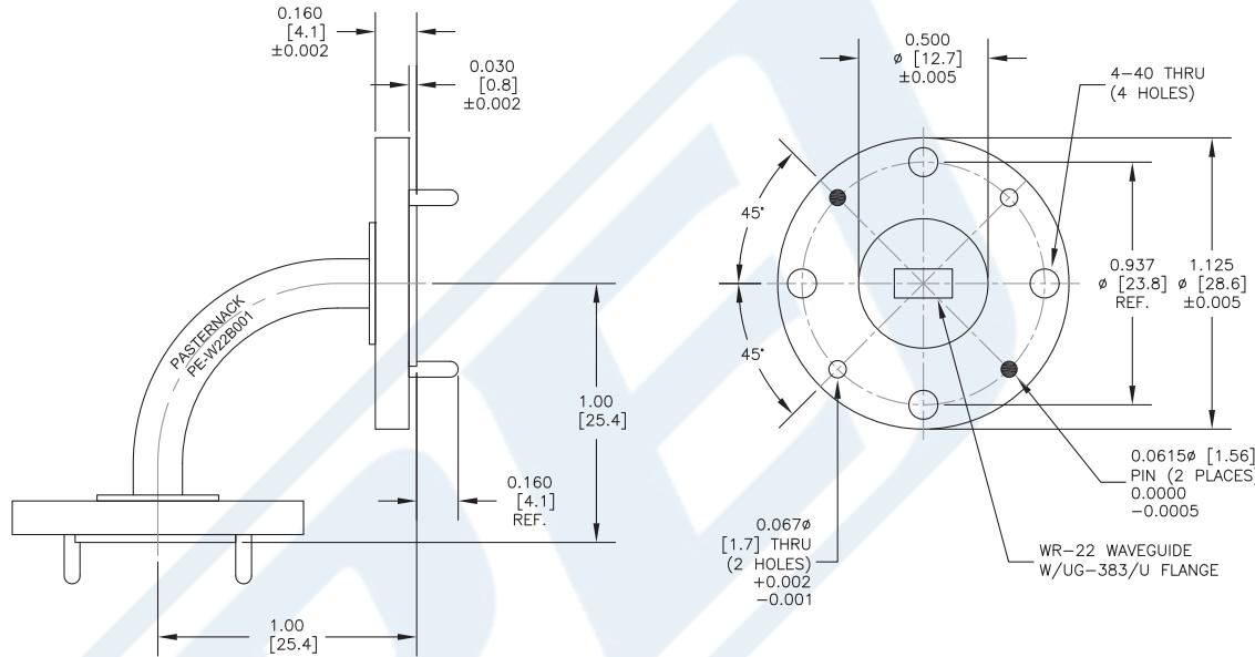
WR-22 Instrumentation Grade Waveguide E-Bend with UG-383/U Flange Operating from 33 GHz to 50 GHz from Pasternack Enterprises has same day shipment for domestic and International orders. Our RF, microwave and millimeter wave products maintain a 99% availability and are part of the broadest selection in the industry.
