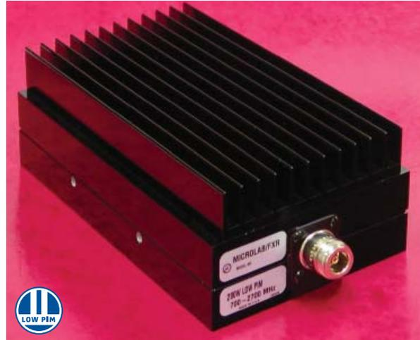
Microlab FP-10 series Cable Attenuators are intended for wireless applications, requiring modest power reduction while maintaining extremely low PIM, (Passive Intermodulation).
