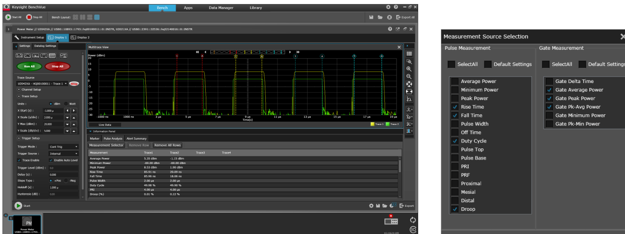
Figure 9. Multi-channel trace display with 4-pairs of gates and automatic pulse parameters measurement (sample screen shot with U2021XA and U2042XA)
