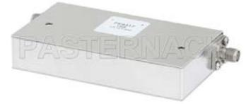
50 Ohm SMA Isolator Operating From 2 GHz to 10 GHz And 10 Watts With 13 dB Isolation
