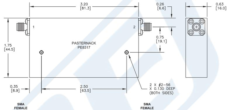
50 Ohm SMA Isolator Operating From 2 GHz to 10 GHz And 10 Watts With 13 dB Isolation from Pasternack Enterprises has same day shipment for domestic and International orders. Our RF, microwave and fiber optic products maintain a 99% availability and are part of the broadest selection in the industry.
