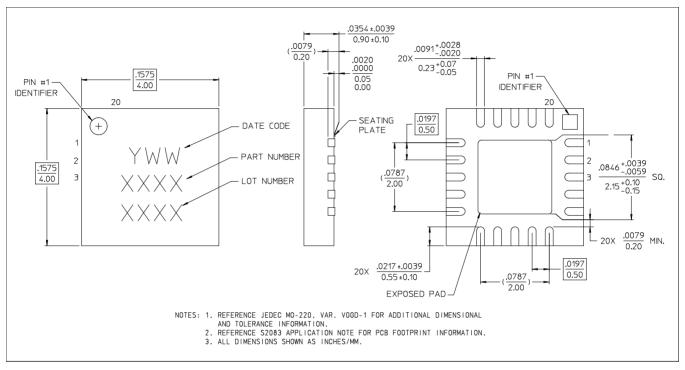
Reference Application Note M538 for lead-free solder reflow recommendations. Plating is 100% matte tin over copper.
