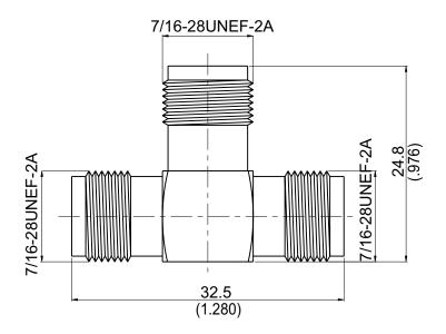
NOTE: 50  $\Omega$  nominal impedance.This connector is a non-matched 3 dB divider for low frequency applications.VSWR  $\geq$  2.0 when terminated 50  $\Omega$ .
