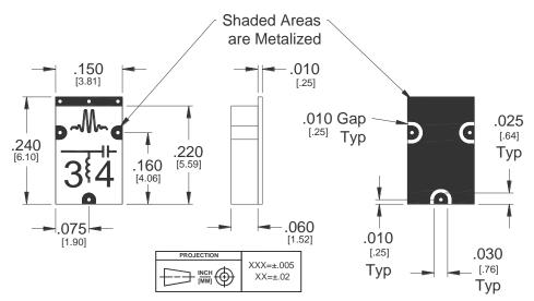
Substrate material is 10-mil thick Rogers 5880 or Taconic TLY-5, ½ Oz Electrodeposited Cu. I/O Pads & Ground Plane Finish is Gold Flash, 5 to 10  $\mu$ -inches, over Solderable Electroless Nickel, 100-200  $\mu$ -inches, over Cu. See <a href="http://www.markimicrowave.com/menus/appnotes/an-btsm-pcb.pdf">http://www.markimicrowave.com/menus/appnotes/an-btsm-pcb.pdf</a> for suggested PCB layout.
