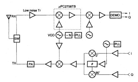
These examples show only IC's location on the system use schematically, do not present or recommend the actual application circuit in detail.
