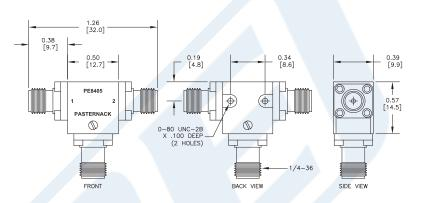
50 Ohm SMA Circulator Operating From 11 GHz to 18 GHz And 10 Watts With 20 dB Isolation from Pasternack Enterprises has same day shipment for domestic and International orders. Our RF, microwave and fiber optic products maintain a 99% availability and are part of the broadest selection in the industry.
