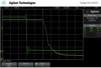
Green Trace = RF Input Pulse Yellow Trace = TTL Output
