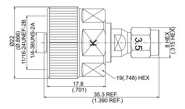
Note:Ruggedized K jack to be mounted directly on vector network analyzer.
