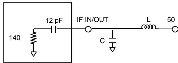
The values of inductance (L) and capacitance (C) are determined by the IF frequency and the length of 50  $\Omega$  line between the package and the LC section. The L & C values for the layout depicted in the sample board layout are listed below for a variety of IF frequencies.
