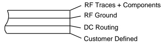
The PCB dielectric between RF traces and RF ground layers should be chosen to reduce RF discontinuities between 50- $\Omega$  lines and package pins. M/A-COM recommends an FR-4 dielectric thickness of 0.008 in. (0.2 mm), yielding a 50- $\Omega$  line width of 0.015 in. (0.38 mm). The recommended metalization thickness is 1 oz. copper.
