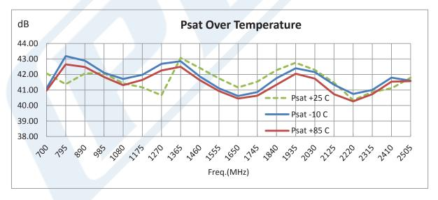
Click the following link (or enter part number in "SEARCH" on website) to obtain additional part information including price, inventory and certifications: 40 dB Gain, 16 Watt P1dB, 800 MHz to 2.5 GHz, High Power High Gain Amplifier, 50 dBm IP3, SMA PE15A5020
