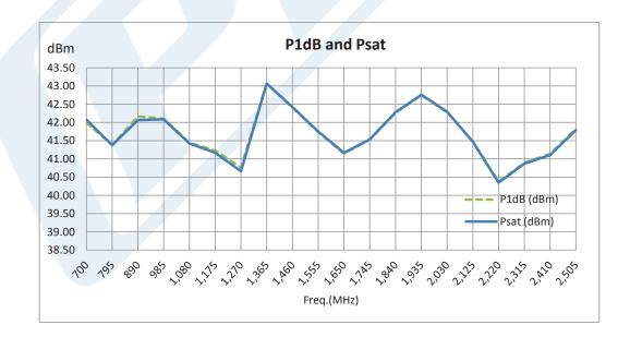
Click the following link (or enter part number in "SEARCH" on website) to obtain additional part information including price, inventory and certifications: 40 dB Gain, 16 Watt P1dB, 800 MHz to 2.5 GHz, High Power High Gain Amplifier, 50 dBm IP3, SMA PE15A5020
